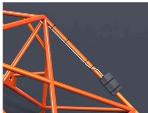
Connecting Cable – routed on inside of roll cage in order to avoid damage in event of car rolling etc.
